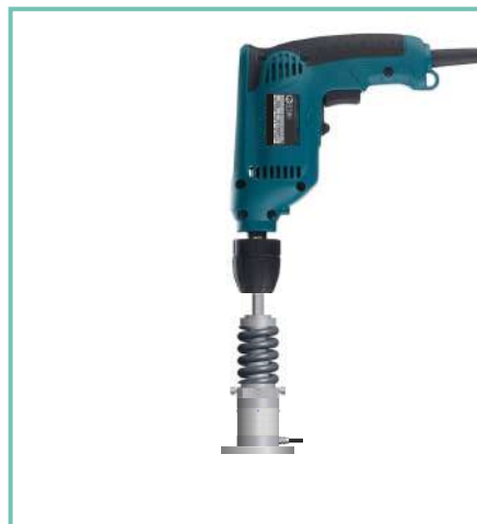
Torque measurement using fidaptor
