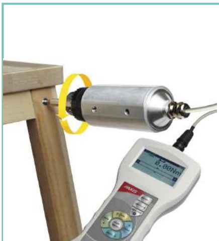
Measurement of the "strength" needed to unscrew
