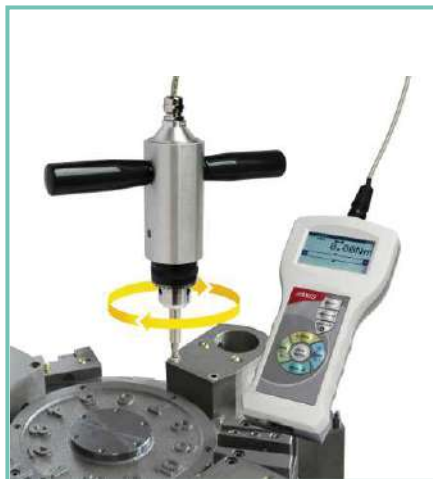
Tightening the screw with precisely defined "strength"
